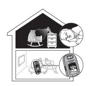
The baby unit has infrared LEDs that allow you to see your baby at night or in a dark room. When the baby unit detects low light levels, the infrared LEDs turn on automatically.
